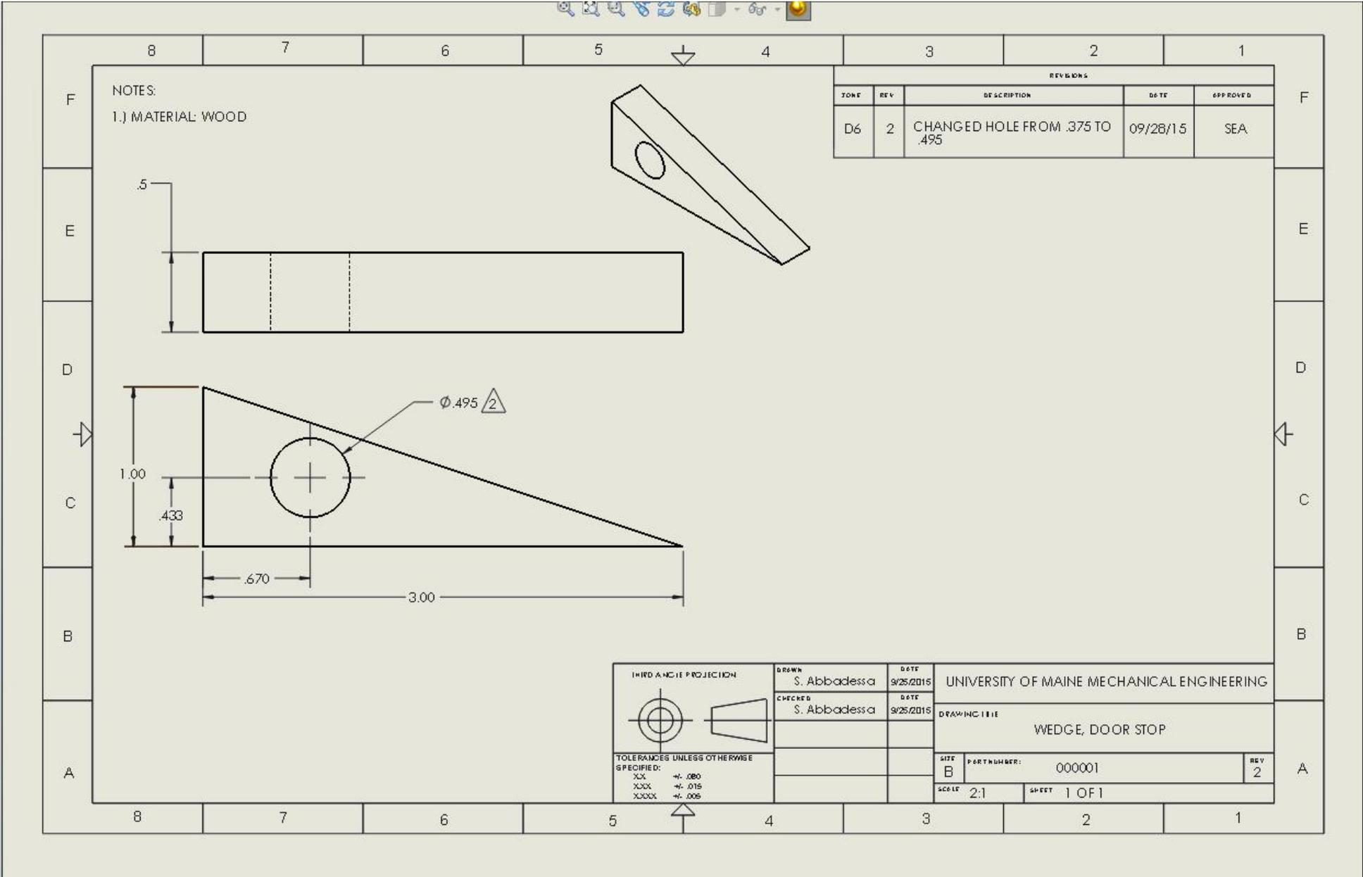
Not all of the six sides of the box need to be shown if the geometry can be fully described with fewer views.
